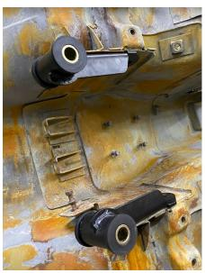
4. Install rear control arm drop-down bracket using OEM hardware. It may be necessary to start one bolt and use a screwdriver to align holes on opposite end.
