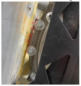
3. Install front diff bracket to car as shown below, using supplied hardware and lock washers. It is also recommended to put some loctite on the threads before install. Do not tighten all the way. Leave loose so the brackets can be slid forward and reverse in slots.
