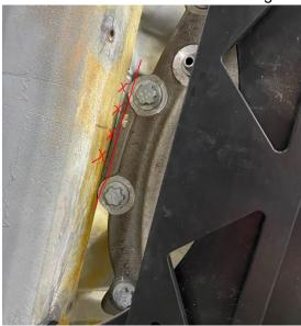
3. Install front diff bracket to car as shown below, using supplied hardware and lock washers. It is also recommended to put some loctite on the threads before install. Do not tighten all the way. Leave loose so the brackets can be slid forward and reverse in slots.
