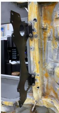
5. Install mustache bar with supplied washers. One washer on top of the bushing, and one on bottom. Reinstall OEM nut hand tight.
